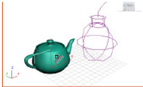
Figure 17-36 The cursor displayed on invoking the Bind to Space Warp tool
