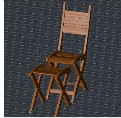
Figure 1-38 The dimetric camera projection
