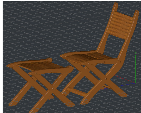
Figure 1-29 The parallel camera projection mode
