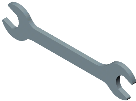
Figure 2-2 Base feature of the spanner
