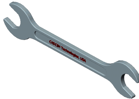
Figure 2-1 Solid model of a spanner
